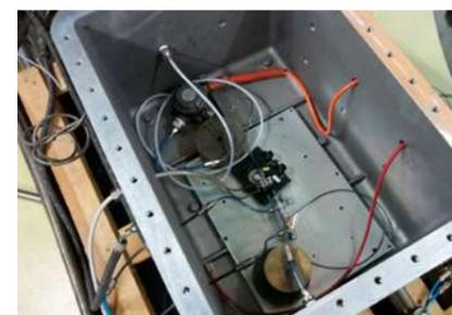
The gas control and mixing system has been designed to realize normative mixtures with oxygen and hydrogen, acetylene, ethylene, propane or methane. The correctness of the mixtures is compared by means of sample mixtures using a gas chromatograph.
