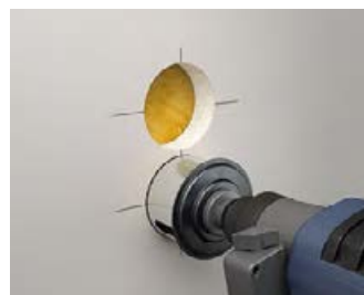
Make Ø 68 mm installation openings with countersinking by using a KAISER cutter (e. g. MULTI 4000 Art. No. 1083-10).
