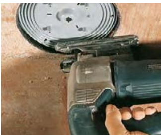
Open front part using a fretsaw.
