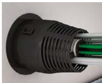
Fit the two-part sealing element round the bundle, close it and connect it to the sealing cylinder by means of the bayonet fitting.
