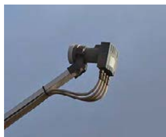
4 coaxial cables are connected here for reception.
