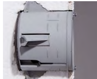
The lip at the back forms a sealing barrier to the insulation material and prevents air draughts along the box.
