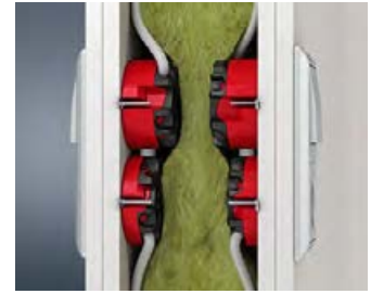
Opposing installation of one-gang boxes in a wall thickness of 100 mm and higher and of one-gang junction boxes in a wall thickness of 125 mm and higher is possible.
