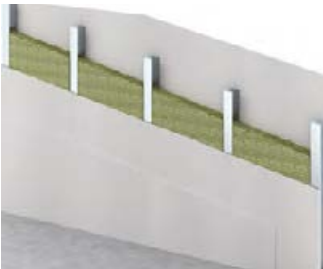
Installation of F90 metal stud walling in compliance with DIN 4102, Part 4
