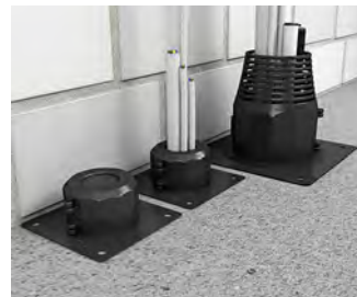
Mixed population of cables and conduits up to maximum population. They can also be arranged as groups with a distance of 205 mm (DS 90 / 120 mm) or 125 mm (DS 90 / 74 mm).
