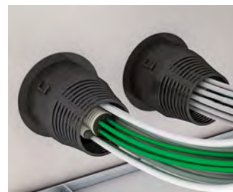
Horizontal alignment of the sealings is possible with a clearance of 50 mm.
