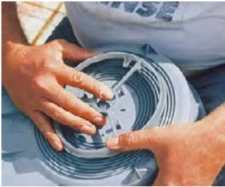
Clip the front ring onto the housing.
