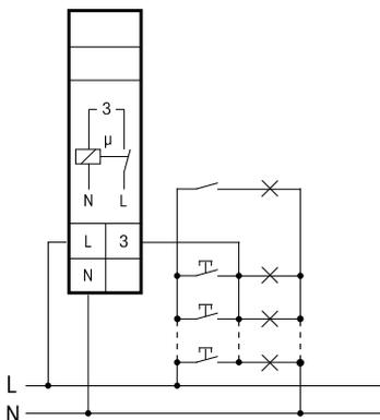
3-wire circuit with attic lighting, not resettable.
