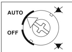
The functions UP and DOWN may be blocked or switched off entirely by a rotary switch. This block applies only to the max.
