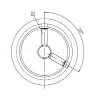
Recommended tolerance of the drive shaft diameter: g6
