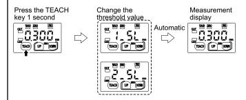
When performing a fine adjustment of the threshold of \$\frac{1}{2} \overline{5} \tau\$ or \$\frac{2}{2} \overline{5} \tau\$, press the UP key or DOWN key. After \$\frac{1}{2} \overline{5} \tau\$ or \$\frac{2}{2} \overline{5} \tau\$ is displayed, the fine adjustment of the threshold can be performed.
