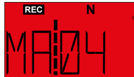
Figure 14: Screen after a circuit breaker trip.
